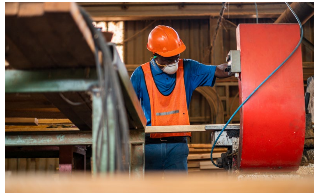
Primary log breakdown (framesaw) in the wetmill department at Timbadola
