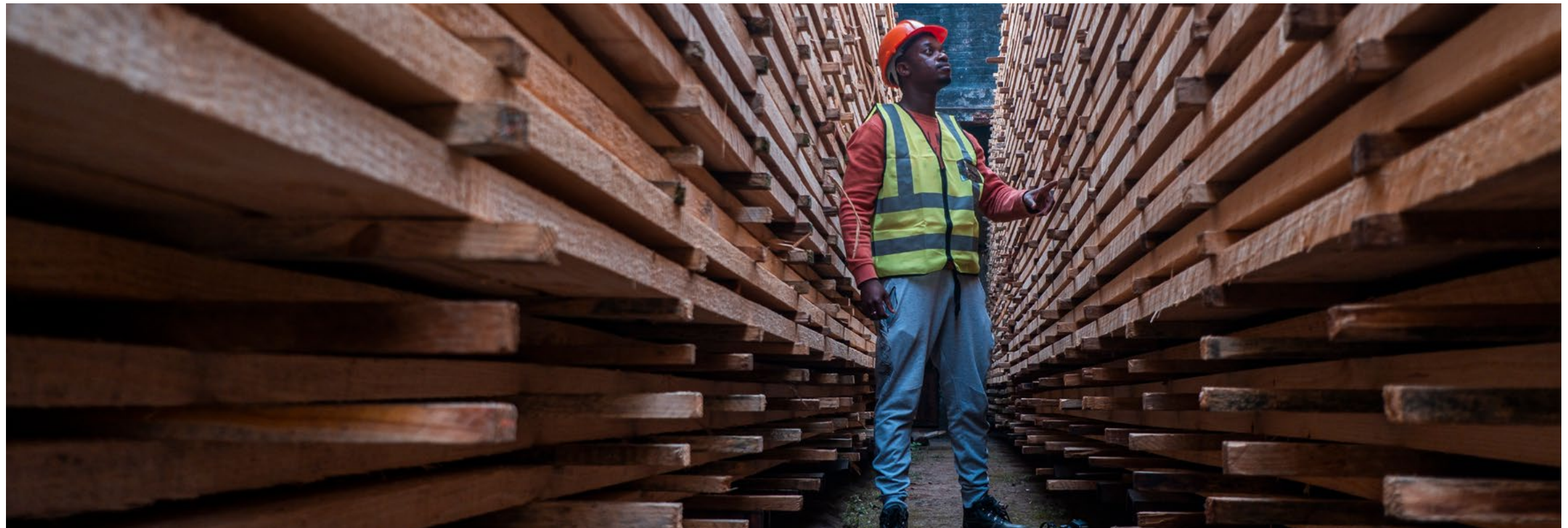
Wet timber stacked on the kiln trolleys for drying at the Timbadola sawmill
