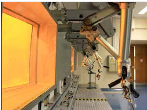
Figure 3: Example of hot cells at a research reactor facility
