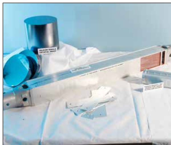
Figure 4: The ingot diameter varies from 128 mm to 152 mm, with a length of 600 mm.
