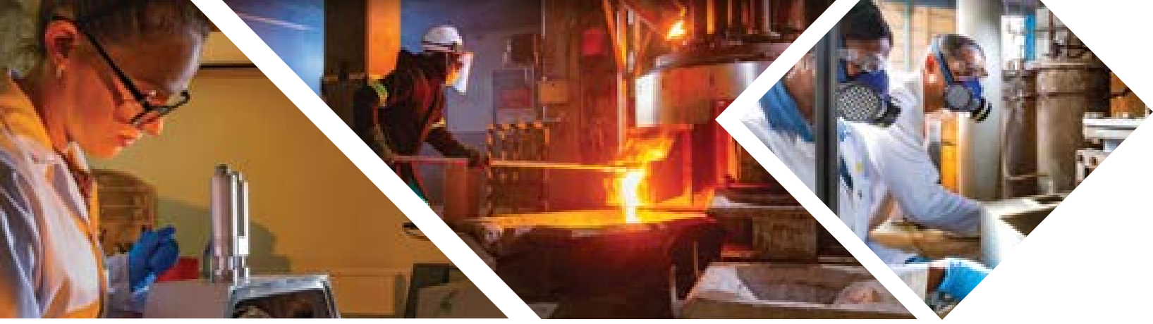
Top left: The QEMSCAN is used in mineralogy division to measure mineralogical variability of materials based on chemistry. Middle: Molten material pours from a DC Arc Furnace during a smelting pilot campaign at Mintek.
