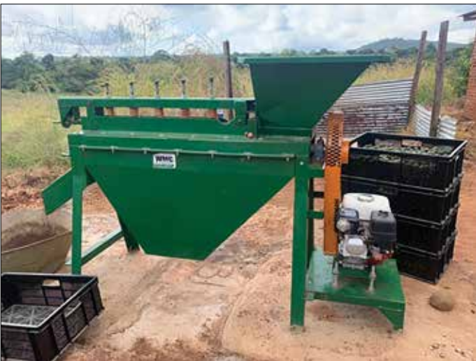
Dehusking machine and harvested macadamia ready for dehusking.
