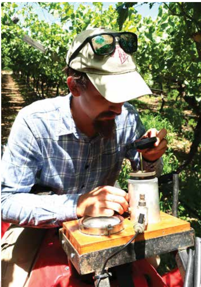
A pressure chamber is used to measure grapevine water status.
