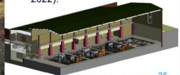
3D Isometric model view of Zuikerbosch Engine Room 2, showing internal layout with engine bays, engines, walkways and stairways
