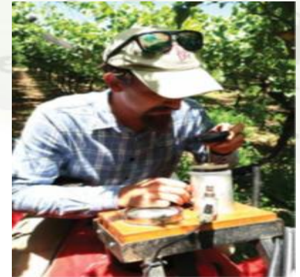
3B A pressure chamber is used to measure grapevine water status.
