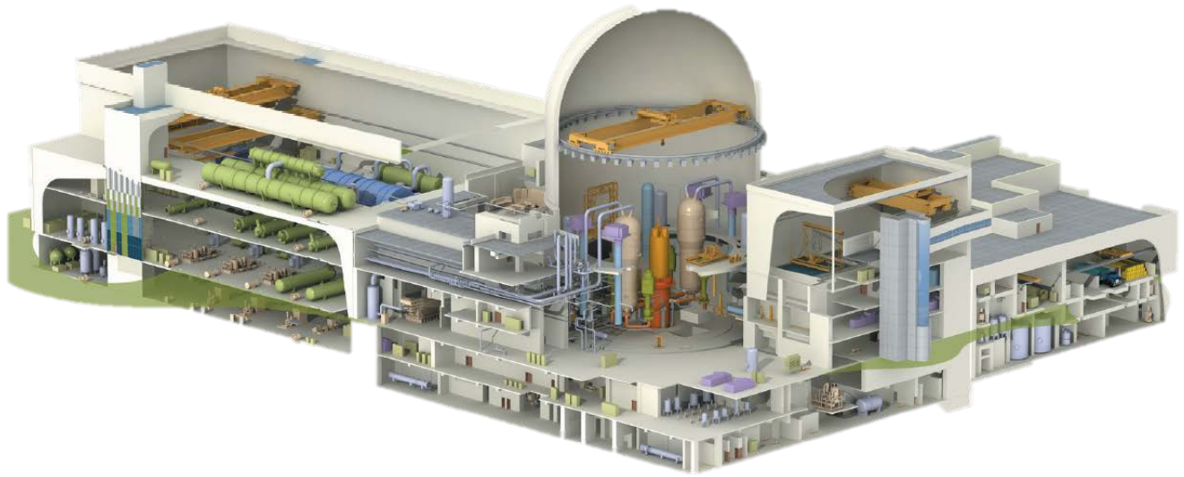
Figure 6-14 APR1400 Plant Layout (02APR1400-Technical Summary-2010.pdf)
