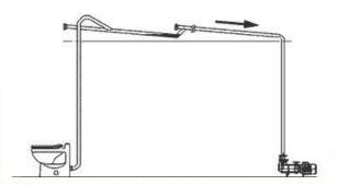
Jets Vacuum Sanitary System is a vacuum sewage collection and transport system designed for single or multiple flushing of toilets. The vacuum toilet system uses air, as opposed to water for the transport of sewage. A Jets Vacuumarator™ evacuates air from the drain pipes automatically upon activation of the activator button.
