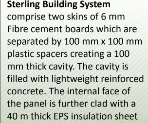
and a 6 mm thick Fibre cement
