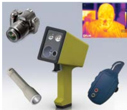
Figure 11: Integrated Thermal Imaging and Acoustic Sounding Device (ITA)
