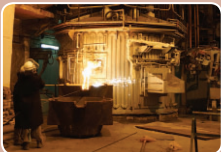
The Atomiser demonstration plant for the water atomisation of alloys.
