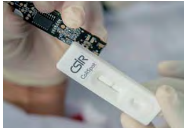
The low-cost E. coli detection device, ColiSpot.
