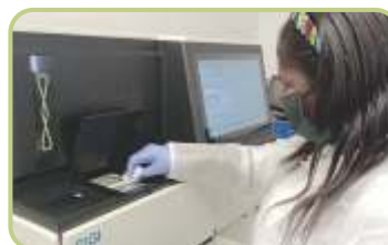
Application Specialist is preparing the MGI DNBSEQ-G400 for a sequencing run.
