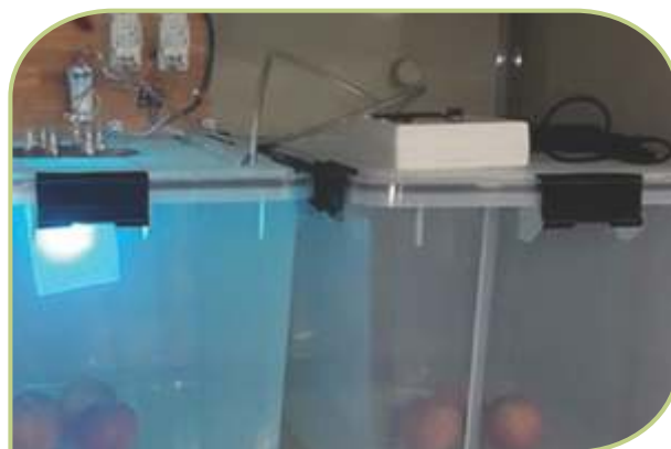
Laboratory trials to compare ethylene removal with VUV photolysis (left) and potassium permanganate adsorbent (right)
